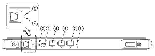
Figure 26. Control processor blade (CP8) LEDs
